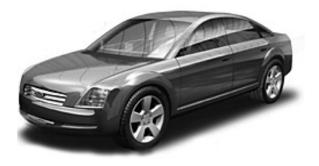
The Ford Prodigy concept, shown in January 2000, achieved 78 MPG using a diesel-hybrid engine and a lightweight, aluminum-intensive body structure. (© 2000 Ford Motor Company)
