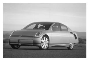
The GM Precept concept, unveiled in January 2000, was designed to achieve 80 MPG with a diesel-hybrid engine and the equivalent of 100 MPG with a hydrogen fuel cell engine. (©2004 General Motors and Wieck Media Services, Inc.)
